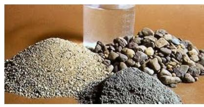
**CONCRETE** is a composite material that consists essentially a binding medium within which are embedded particles of aggregate
